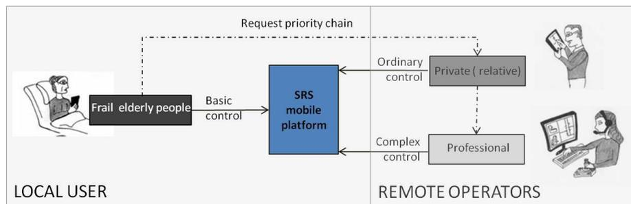
**Fig. 4.** The developed concept of SRS [2]. The figure shows the users of the systems, the idea of three different devices with increasing complexity that they should use to interact with the robot or with the other stakeholders, and the priority chain of intervention.
