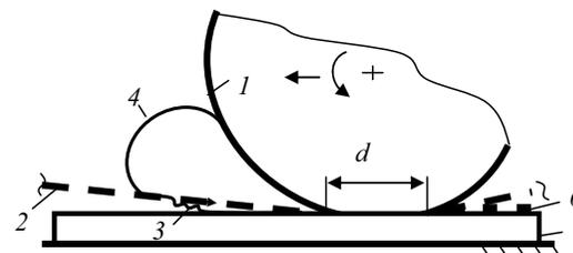
Fig. 1. The scheme of ink current in a working layer:
