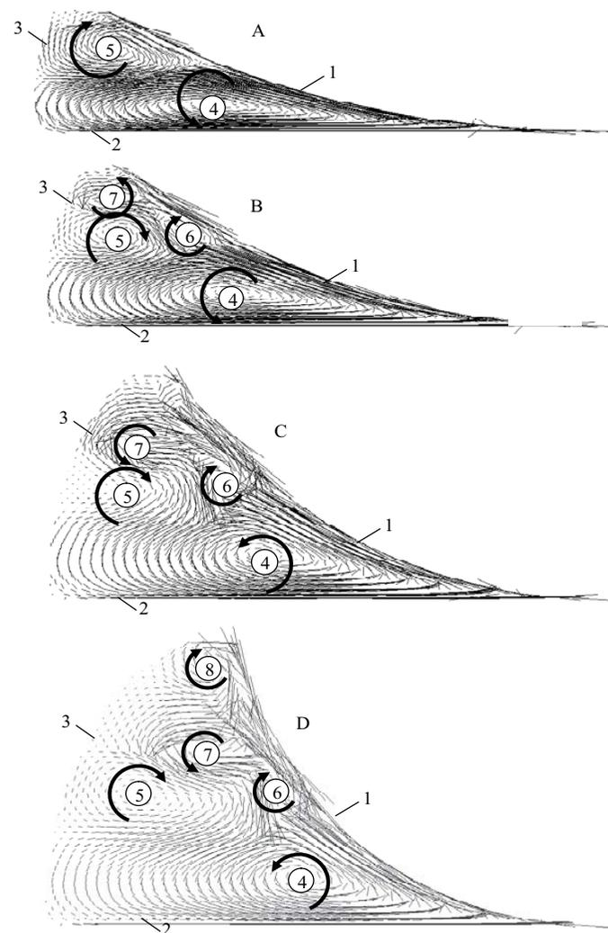
Fig. 3. Change of a field of speeds depending on a corner defining quantity of a paint in a working layer: A –  $\alpha=30^\circ$ ; B –  $\alpha=40^\circ$ ; C –  $\alpha=60^\circ$ ; D –  $\alpha=80^\circ$ ; 1 – a surface of the cylinder; 2 – a plane качения the cylinder; 3 – a free surface; 4, 5, 6, 7, 8 – whirlwinds
