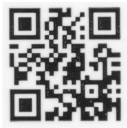
Abbildung 8: QR-code with module size 0.5 mm printed in Flexo, original image
