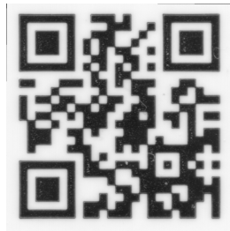
Abbildung 9: Module size 0.5 mm printed in Flexo; rotated
