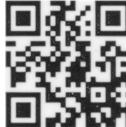
Abbildung 10: Modul size 0.5 mm printed in Flexo
