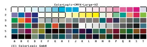
Pic 6: Mini Colour Management Test Target by ColorLogic
