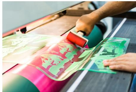
Pic 5: Mounting of a Flexo printing plate
