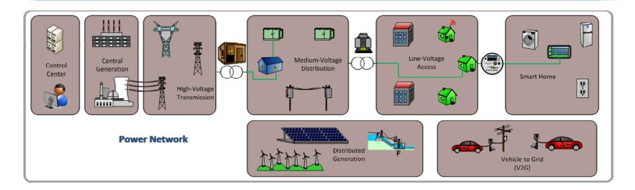
CC-IIMSN definition: Smart Grid means that different electrical grid elements must now exchange data with the "outside world" > a communication system is required.
