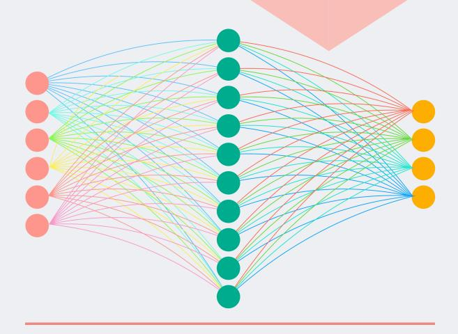
The input layer is comprised of five nodes, each representing the car's distance to the edge of the track, along with one neuron dedicated to acceleration. Additionally, the network includes a hidden layer featuring 10 neurons and an output layer with 4 neurons representing the possible actions the network can undertake: acceleration, braking, right-turning, and left-turning.
