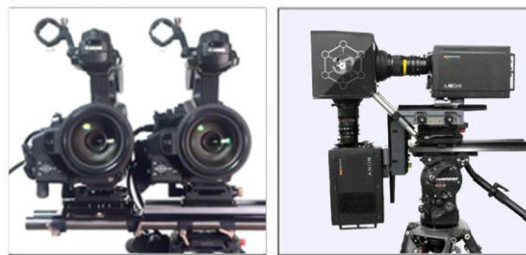
Figure 60: Left: side-by-side rig, right: beam-splitter rig.
