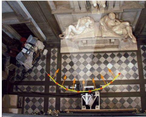
Figure 66: To generate a light field of a static scene, a single moving camera capturing various perspectives is sufficient.
