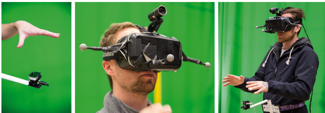
Fig.23: RET-VP prototype: (left to right) Leap Motion controller, Oculus Rift with webcam, complete setup
