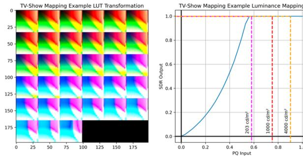
Figure 4: LUT image and transfer function of the TV-Show Mapping Example
