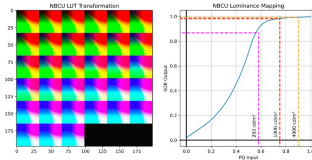
Figure 6: LUT image and transfer function of the 5 NBCU PQ2SDR LUT
