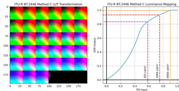
Figure 3: LUT image and transfer function of ITU-R BT.2446-1 Method C
