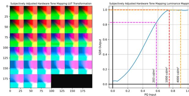
Figure 5: LUT image and transfer function of the Subjectively Adjusted Hardware Tone Mapping
