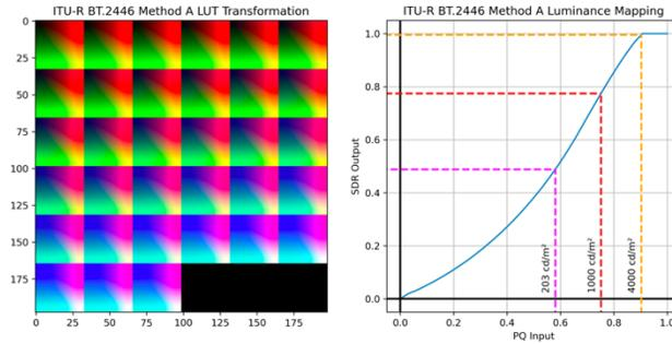
Figure 2: LUT image and transfer function of ITU-R BT.2446-1 method A
