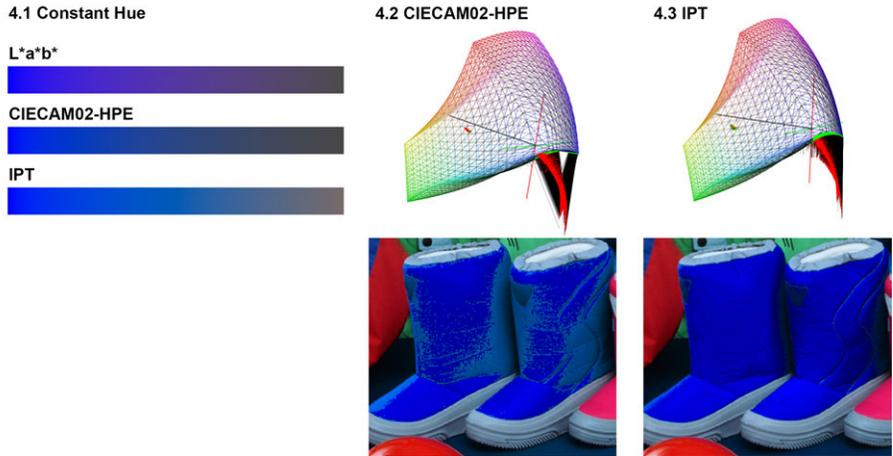
Figure 4. Artifacts introduced by the color space in which the gamut mapping is performed. 4.1 shows bluish colors of different lightness, constant hue and increasing saturation predicted by L\*a\*b\*, CIECAM02-HPE and IPT. In Figure 4.2 a detail from the ISO 165 "Ski" test image<sup>6</sup> is presented along the corresponding 3D-rendering of gamut mapping this image via mindE to sRGB<sup>19</sup> color space.
