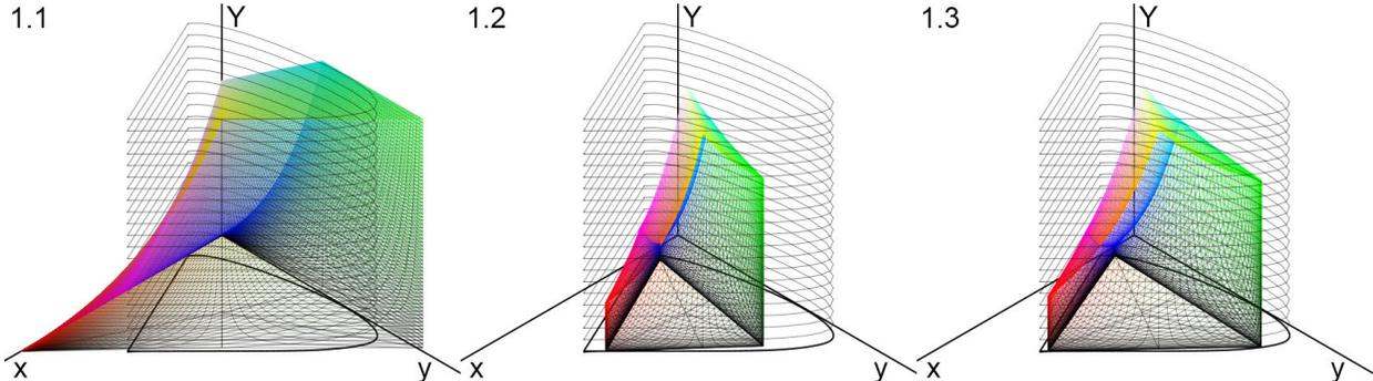
Figure 1. DCI X'Y'Z' color space (1.1) compared to DCI reference projector gamut "P3ref" (1.2) and the gamut of a prototype laser projector "P3laser" (1.3) from the OSIRIS project<sup>3</sup>. The lower axes x and y are the CIE 1931 chromaticity diagram x- and y-axes, the vertical axis is the Y-component of the CIE 1931 2° standard observer.
