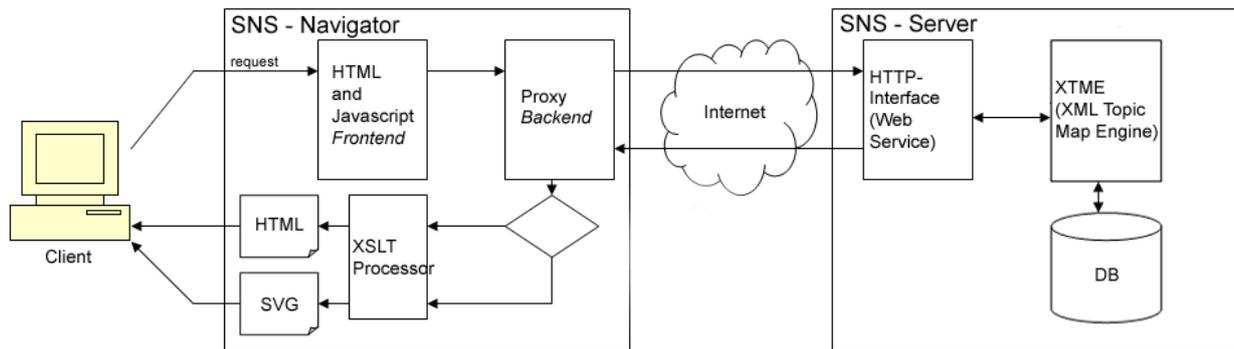
**Figure 6:** Three-tier architecture of the SNS-Navigator web application
